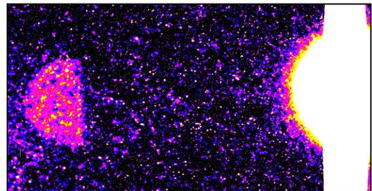
Fig. 5: Diffracted signal from InSb crystal. The beam on the left is the Bragg diffracted signal from the crystal. The beam on the right is the main x-ray pulse, saturated CCD.
