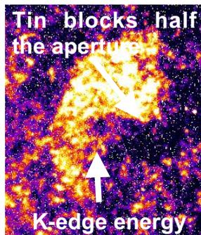
Fig. 6. Diffracted x-rays from InSb. Sn is used to filter the bottom half of the x-ray pulse. The x-rays were tuned so that the high energy x-rays would be absorbed by the Sn, leaving the diffracted signal with a sharp high energy edge.
