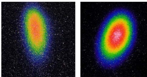
Fig. 3a.: X-rays generated from the velocity compressed, 300fs, electron beam vs. (b) uncompressed 5 ps beam.
