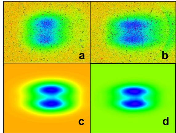
Fig. 4: K-edge radiography through U. 4a. PLEIADES tuned to 115 keV k-edge, for on axis x-rays, which are absorbed by k-edge. 4b. PLEIADES tuned away from k-edge, on axis x-rays begin being transmitted through foil. 4 c and d are BLOWER simulations.
