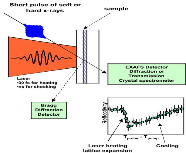
Fig. 1. Schematic of laser-x-ray pump probe
