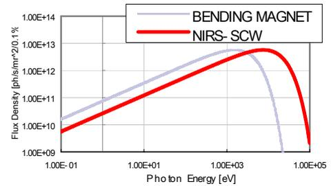
Figure 1: Spectra of the SCW and the bending magnet at SAGA-LS.
