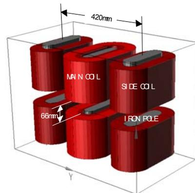
Figure 2: Field calculation model of the SCW.
