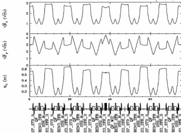
Figure 7: Beta and dispersion functions after tune correction. The SCW position is center of the lattice.
