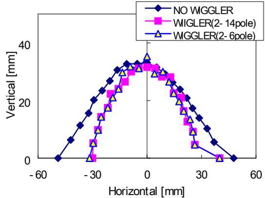
Figure 8: Dynamic aperture at center of the long strait section. Tracking turn number is 25000, which corresponds to damping time at 1.4 GeV.
