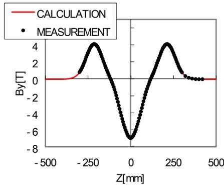
Figure 3: Calculation and measurement of the SCW vertical magnetic fields.
