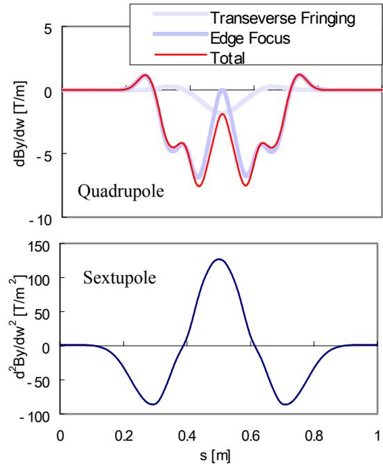
Figure 6: Quadrupole (up) and Sextupole (down) distributions along beam orbit. Quadrupole is decomposed to two contributions due to the SCW transverse fringing field and edge focus.
