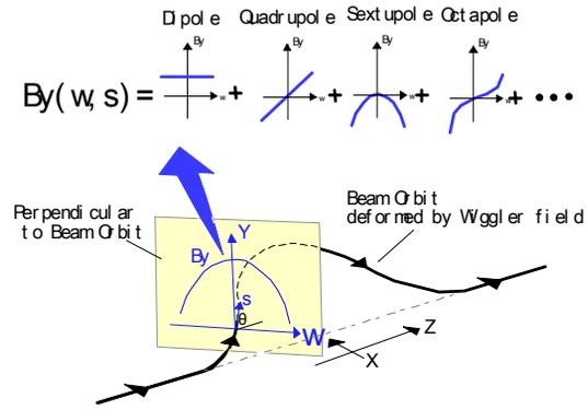
Figure 5: Schematic view of multipole expansion along beam orbit.
