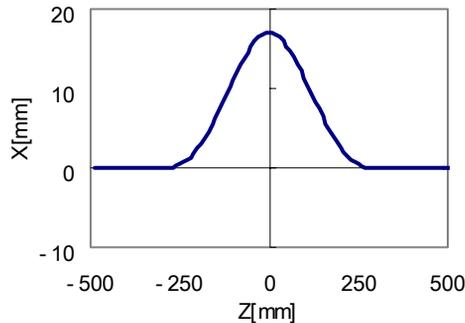
Figure 4: Beam orbit in the SCW section. Horizontal and vertical axis show the longitudinal and transverse direction on the design orbit, respectively.
