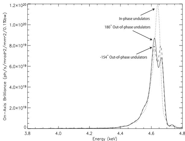
Figure 1: On-axis brilliance of the first harmonic for two undulators in series at an undulator gap of 13.5 mm ( $K = 2.02$ ). The dotted line is for perfectly phased undulators, and the solid line is for undulators 180° out of phase. The dashed line shows the performance for a -154° phase shift, which represents the worst case. The brilliance is reduced to 73% / 66% (at the peak; solid and dashed line) of the brilliance for in-phase undulators.
