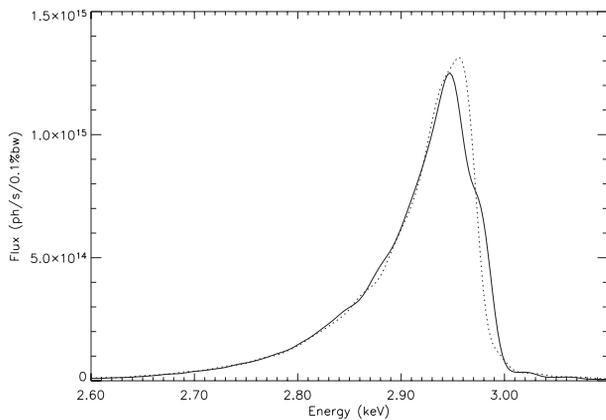
Figure 3: Flux through a 2.0 mm (h) x 1.0 mm (v) aperture at 30 m (first harmonic) for two collinear undulators at 10.5 mm gap ( $K = 2.74$ ) with the APS beam emittance and beam energy spread taken into account. The dotted line is for perfectly phased undulators, and the solid line is for undulators  $180^\circ$  out of phase.
