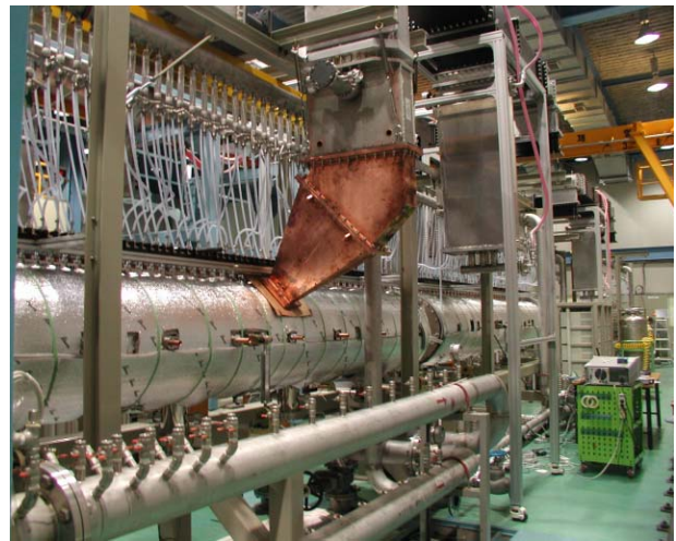
Figure 9: DTL tank1, tank2 under tuning.
