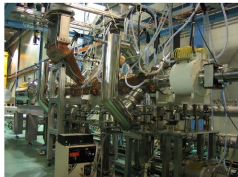
Figure 5: The PEFP RFQ and its test stand.
