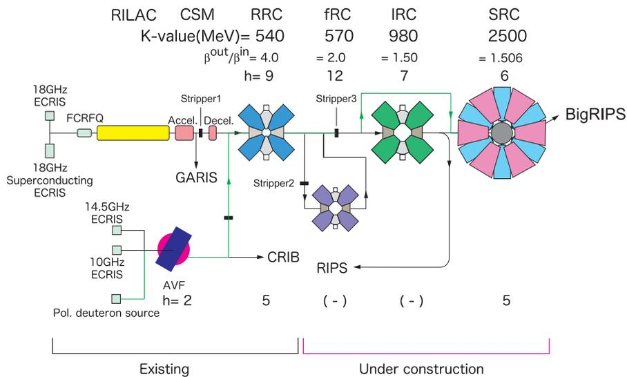
Figure 2: A schematic diagram of the RIBF heavy-ion accelerator system.
