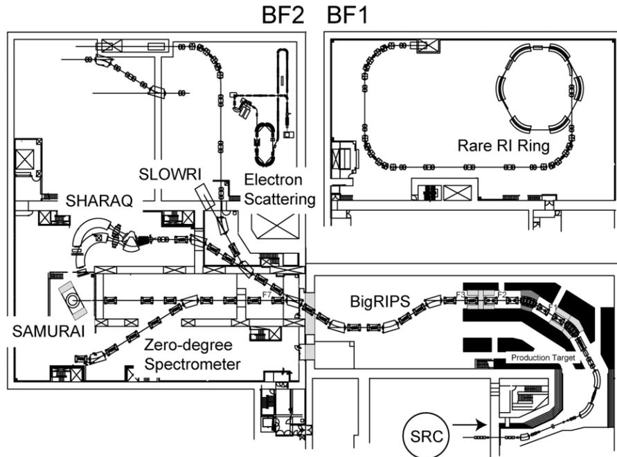
Figure 7: Layout of the BigRIPS and the major experimental installations planned in the second phase.
