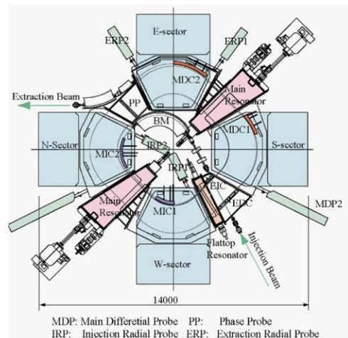
Figure 5: Layout of the IRC.
