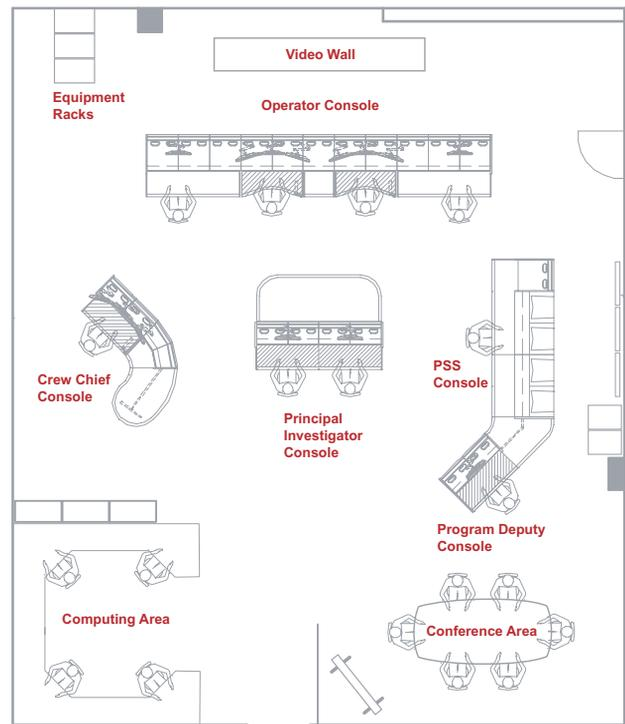
Figure 7: New control room layout.
