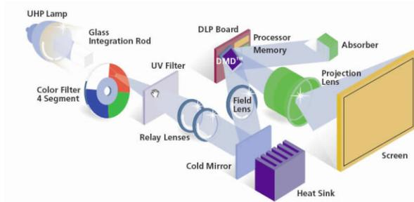
Figure 8: Display Wall projection engine.
