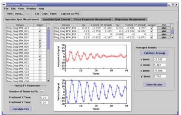
Figure 7: The Ring injection application, being developed using simulated signals from the virtual accelerator.
