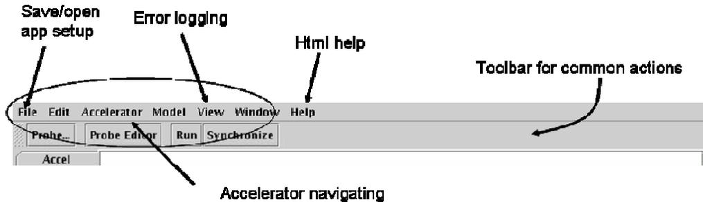
Figure 3: The XAL GUI application framework view, showing common features inheritable by all applications.
