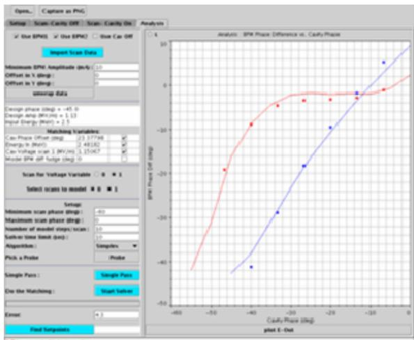
Figure 5: A PASTA application screen shot, showing a comparison of model (dots) and measured lines (BPM) phase differences.
