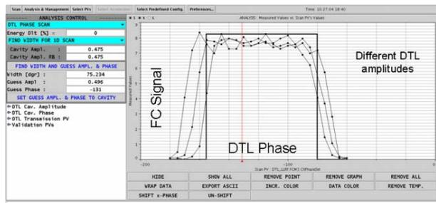
Figure 8: The scanning application screen shot, showing an example where RF phase was scanned at different amplitudes and a Faraday Cup signal was measured.
