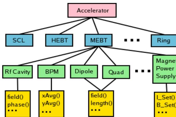
Figure 2: Schematic of the XAL accelerator class hierarchy.
