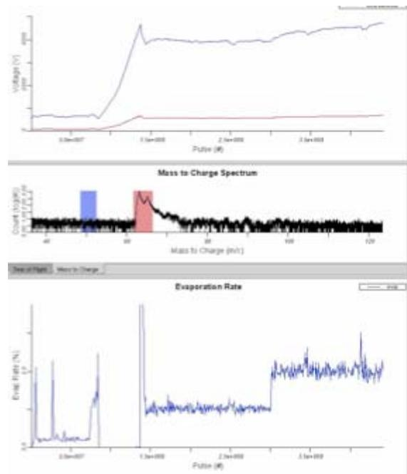
Figure 3: A screen shot of V, m/q and evap. rate for Cu.
