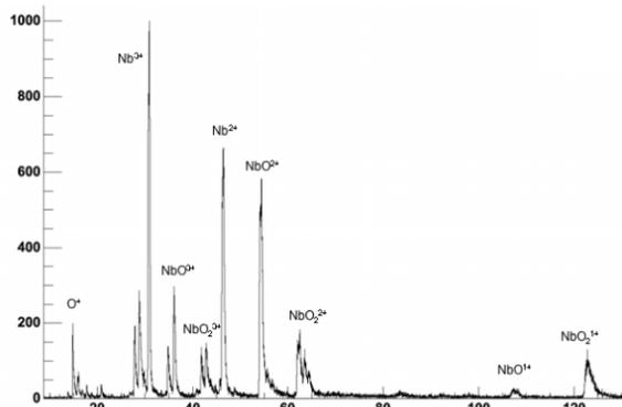
Figure 5: Ions initially field evaporated from niobium.
