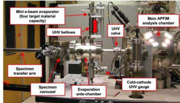
Figure 6: The coating test assembly.
