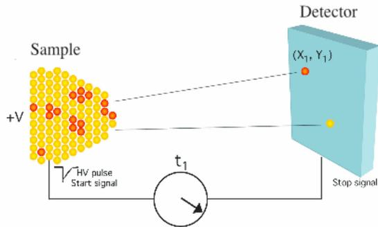
Figure 2: The principle of the atom probe tomography
