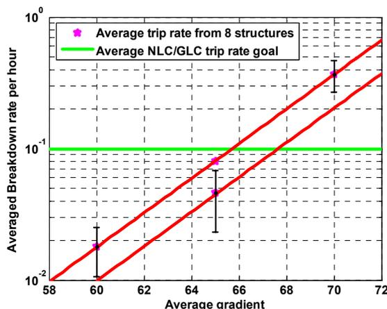
Figure 3: Average breakdown rate as a function of accelerating gradient.
