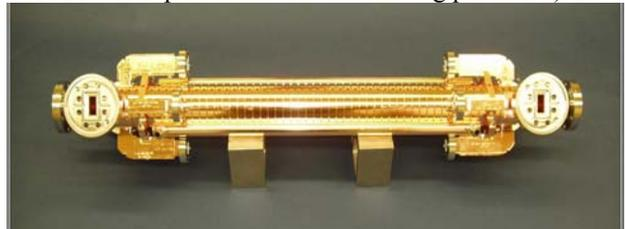
Figure 1: NLC accelerating structure with power couplers and HOM couplers on each side.
