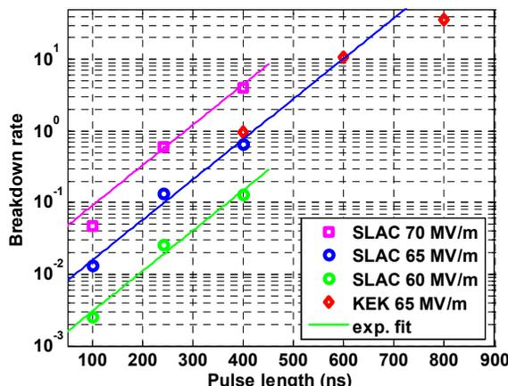
Figure 4: Pulse length dependence of the breakdown rate.
