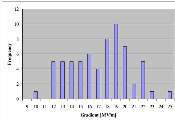
Figure 4: Distribution of maximum gradients achieved in the SNS superconducting cavities so far (65 out of 81) at 4.2 K in open loop at 1.3 msec pulse length at 10 pps. The overall average value is 17.8 MV/m.
