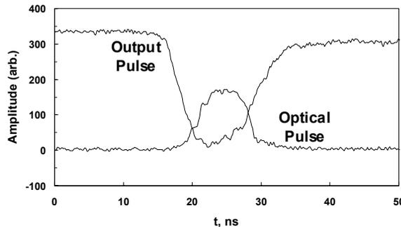
Figure 7. SiC switch. Output (top), optical pulse (bottom)
