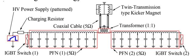
Figure 7. Main schematic of J-PARC main ring extraction fast kicker.
