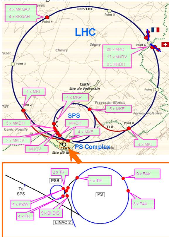
Figure 4. Fast pulsed magnet systems in the LHC chain
