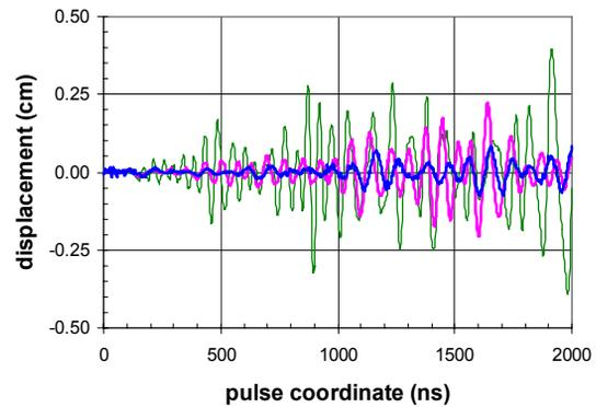
Figure 5: Horizontal beam displacement along the pulse when uniform radii of 0.445, 0.668, and 0.890 cm (green, red, and blue) are used over the transport channel.
