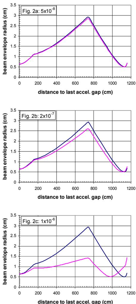
Figure 2: Beam envelopes for the head (blue) and for the tail (red) between the last accelerator gap and the septum quad at different pressure.
