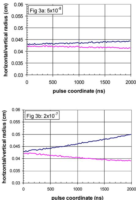
Figure 3: Horizontal (red) and vertical (blue) beam radii during the beam pulse at the final focus for pressure levels (a)  $5 \times 10^{-8}$  and (b)  $2 \times 10^{-7}$  torr.
