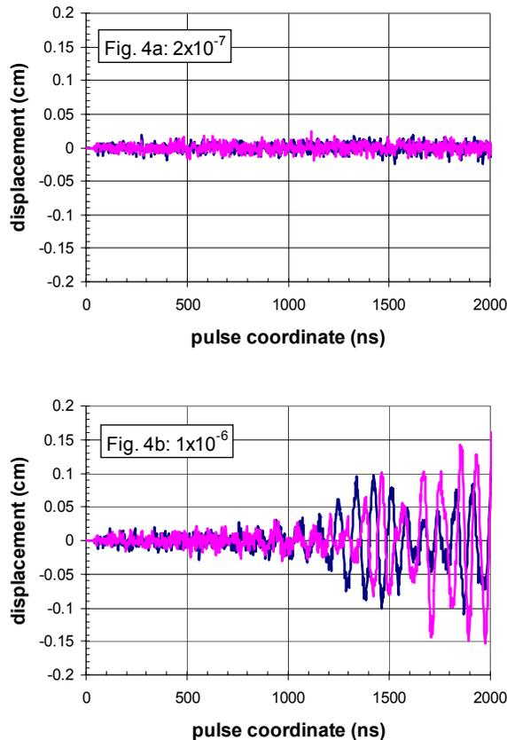
Figure 4: LSP results of horizontal (red) and vertical (blue) beam displacement, observed at the septum quad, due to ion-hose effect at pressure levels of (a)  $2 \times 10^{-7}$  and (b)  $1 \times 10^{-6}$  torr.
