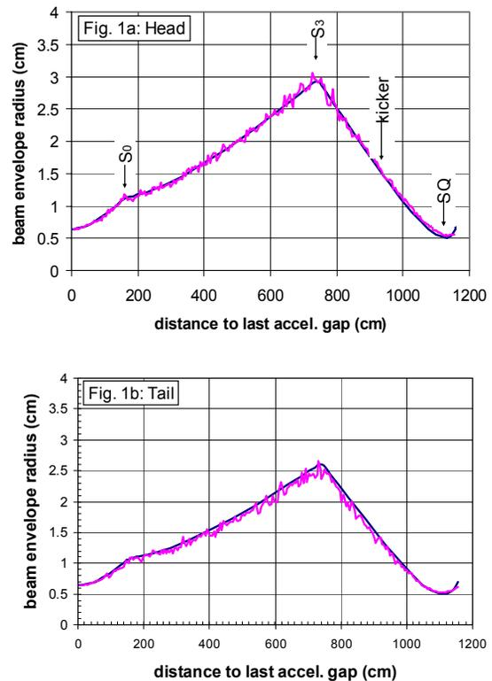
Figure 1: Comparison of beam envelopes calculated using LAMDA (blue) and LSP (red) at  $2 \times 10^{-7}$  torr for the head (a) and the tail (b) of the pulse. Locations of the magnetic transport elements  $S_0$ ,  $S_3$ , kicker, and septum quad (SQ) are also marked in Fig. 1a.
