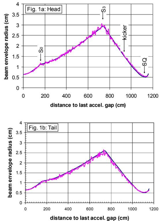
Figure 1: Comparison of beam envelopes calculated using LAMDA (blue) and LSP (red) at  $2 \times 10^{-7}$  torr for the head (a) and the tail (b) of the pulse. Locations of the magnetic transport elements  $S_0$ ,  $S_3$ , kicker, and septum quad (SQ) are also marked in Fig. 1a.
