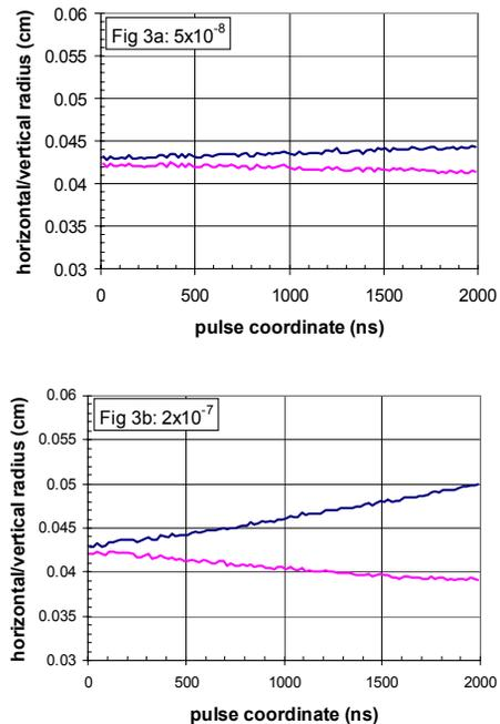
Figure 3: Horizontal (red) and vertical (blue) beam radii during the beam pulse at the final focus for pressure levels (a)  $5 \times 10^{-8}$  and (b)  $2 \times 10^{-7}$  torr.
