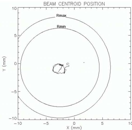
Figure 4: Beam position at accelerator exit during a 400 ns window around peak current compared with estimated beam size from XTR envelope code for a probable range of initial conditions. (S and F signify start and finish of trajectory).
