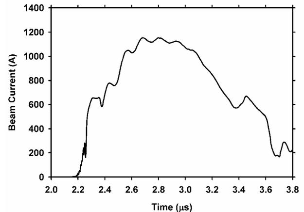
Figure 2: 1200-ns FWHM beam pulse at exit of accelerator in initial experiments (configuration A).
