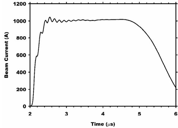
Figure 5: Injector current waveform for a long-pulse test shot.
