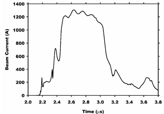
Figure 3: 800 ns FWHM beam pulse at exit of accelerator in initial experiments (configuration B).
