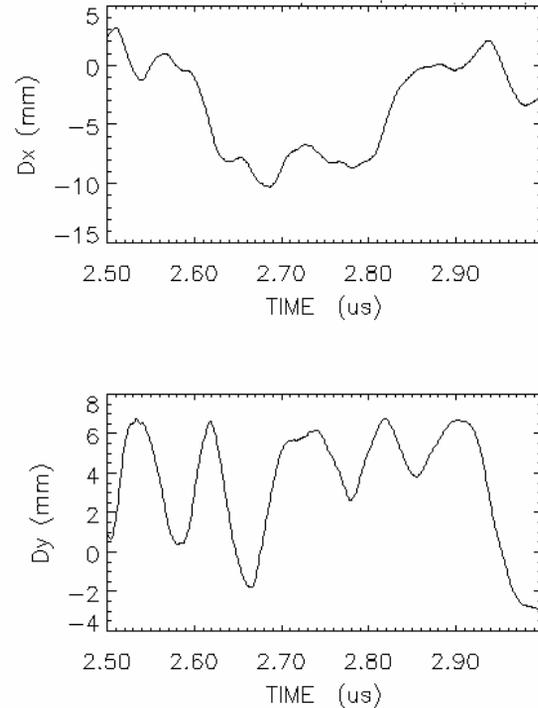
Figure 7: Beam motion at the entrance to the last cell block showing the 10 to 12 MHz ion-hose motion. (The 7.8 MHz oscillation has been filtered out of these data.)
