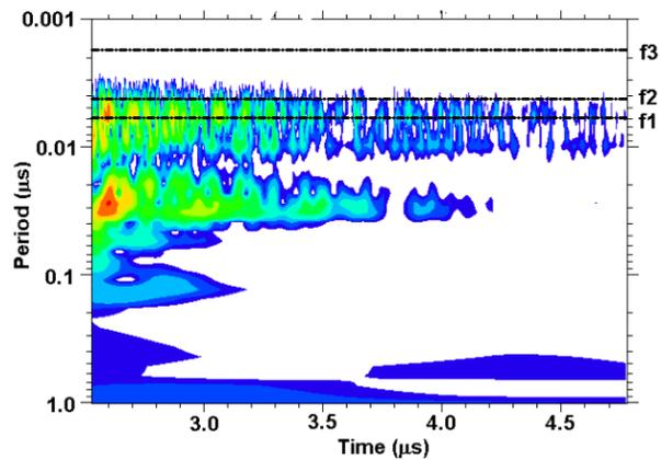
Figure 6: Frequency analysis of  $dy/dt$  during 2 ms flat top of current pulse. (The 7.8 MHz oscillations were filtered out for this analysis.)
