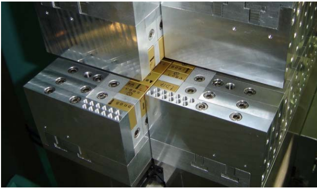
Figure 5: Undulator end-section showing the holder for the small correcting permanent magnet pieces.
