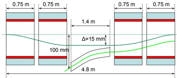
Figure 4: Short injection straight.
