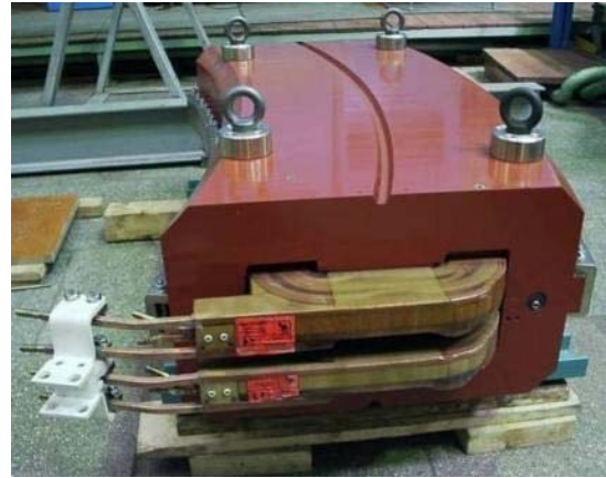
Figure 1: Booster dipole at BINP ready to ship to Duke.
