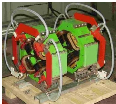
Figure 2: Quadrupoles at BINP ready to ship to Duke.
