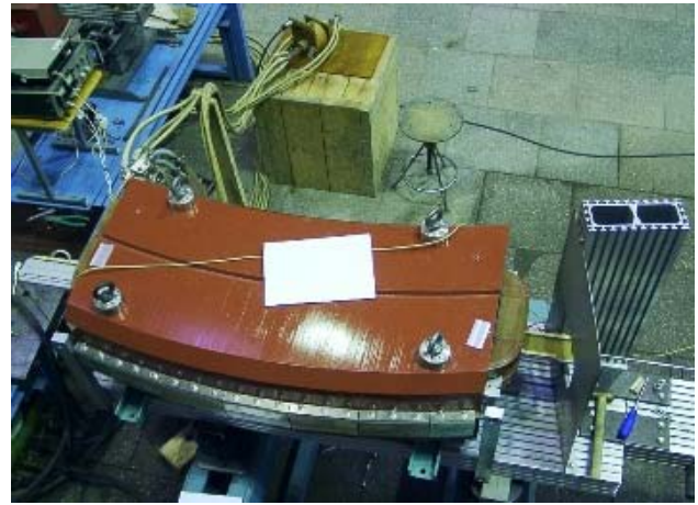
Figure 3: Magnetic measurement set-up for the dipoles.
