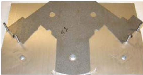
Figure 3: The original 1/16-inch thick CESR quadrupole steel lamination.
