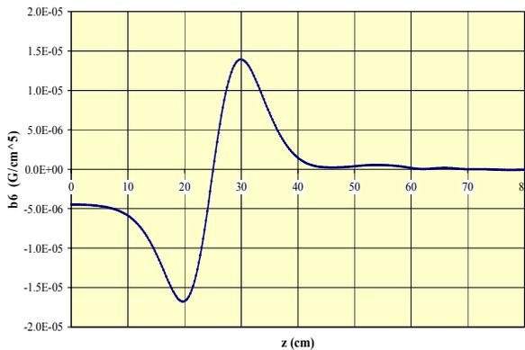
Figure 5: Generalized gradient  $b_6$  vs.  $z$  for 30Q58.
