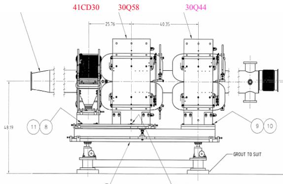
Figure 1: SNS ring doublet assembly [4].
