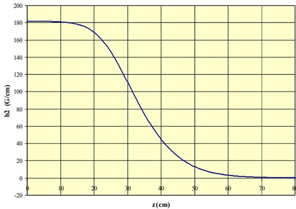
Figure 4: Linear gradient  $b_2$  vs.  $z$  for 30Q58.
