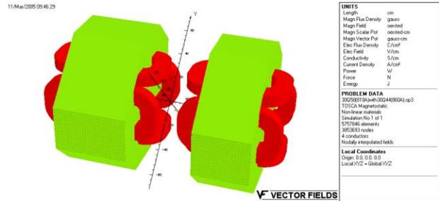
Figure 6: Simulation model for two doublet magnets.
