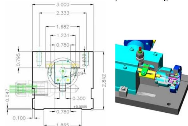
Figure 2: Cross-section in central region. Dimensions are at the left. Oil comes out through the tube connected to the space below G10 rods painted yellow, right.
