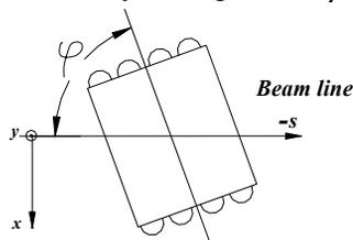
Figure 3: Single octupole/quadrupole/... tilted by angle  $\phi$  in horizontal plane. The tilt can be arranged in vertical plane as well.
