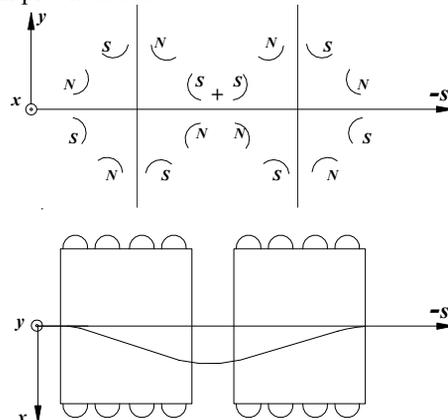
Figure 2: Octupoles installed rectangular to the beam trajectory. Trajectory is shown also. It runs ~in central part of each octupole ~along axis  $-s$ . For these purposes the yoke must have side openings there.
