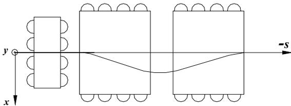
Figure 5: Combination of defocusing octupole and octupole wiggler (pair of octupoles installed normally to the beam's trajectory) with appropriate orientation ( $x/y$ ) can be focusing/defocusing in any direction.
