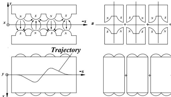
Figure 1: Ordinary dipole wiggler can be represented as series of *quadrupoles* oriented transversely. Horizontal plane of this dipole wiggler can be oriented vertically as well. Particles are moving along  $-s$ .
