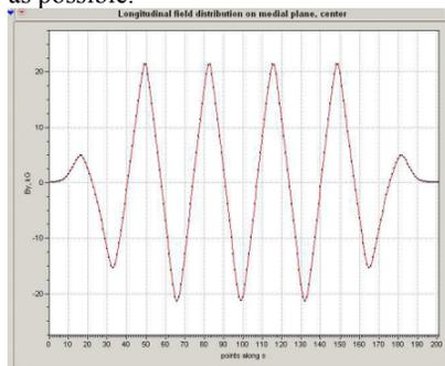
Figure 5: Longitudinal field dependence (as function of  $s$ ) at  $x=0$  calculated for wiggler Fig. 3 with tapering ~1/4, 3/4, 1. Right point on this picture corresponds to  $s=150$  cm.
