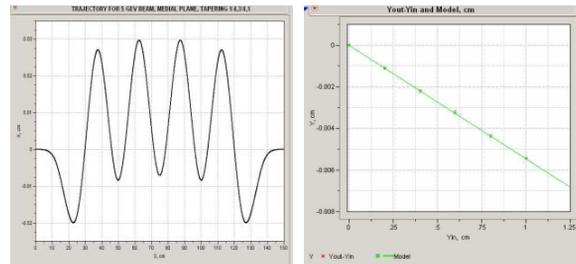
Figure 6: Trajectory of electron with energy 5 GeV entering at  $x=y=0$ , left. Difference between exit and entrance  $y$ -coordinates and the linear model fit, right.
