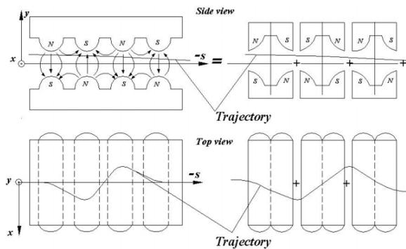
Figure 1: Representation of wiggler as series of quadrupoles with *transverse* orientation.
