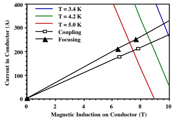
Figure 4. The MICE focusing and coupling magnets load lines in the flip mode. (The higher current points are  $p = 240$  MeV/c; the lower current points are for 200 MeV/c.)
