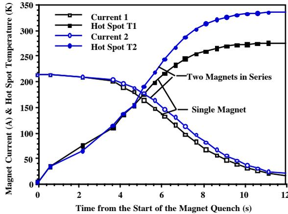
Figure 4. The coupling magnet current and hot spot temperature as a function of the time from the quench start for a single magnet and two magnets connected in series.
