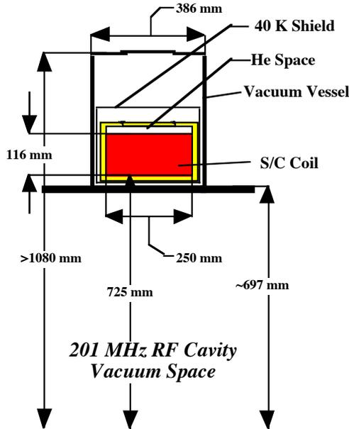
Figure 3. A cross-sectional view of one half of the coupling magnet showing the magnet dimensions
