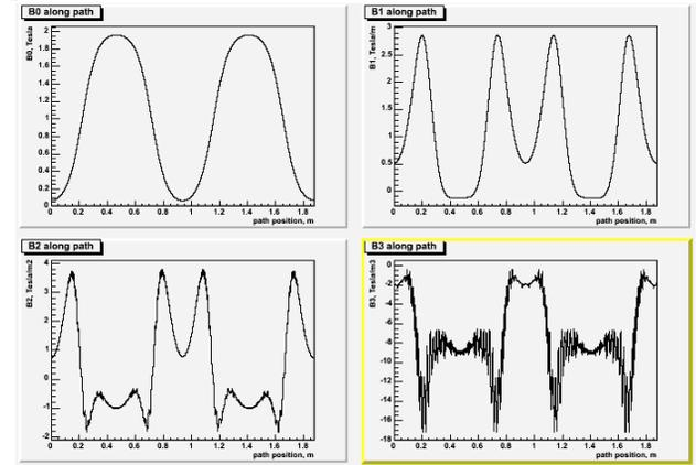
Figure 4: Field harmonics along the closed orbit path.
