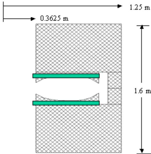
Figure 2: Vertical cross section of the magnet along the symmetry plane.
