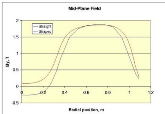
Figure 3:  $B_y$  in the mid-plane of the vertical symmetry plane. The red curve shows the field with the shape pole. The blue curve shows the field for flat poles.
