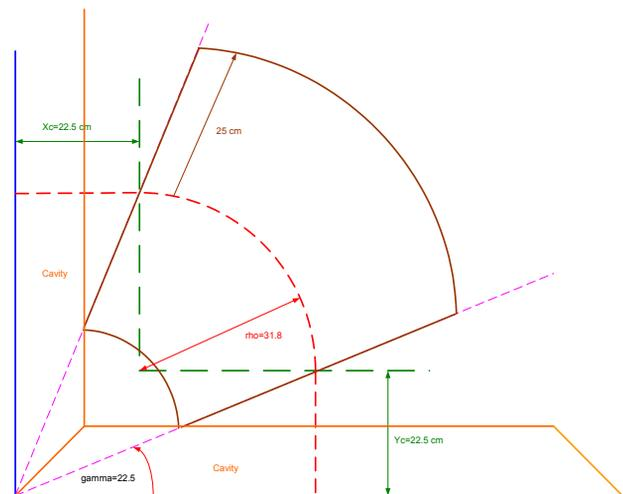
Figure 1: Sketch showing a single cell of the cooling ring.
