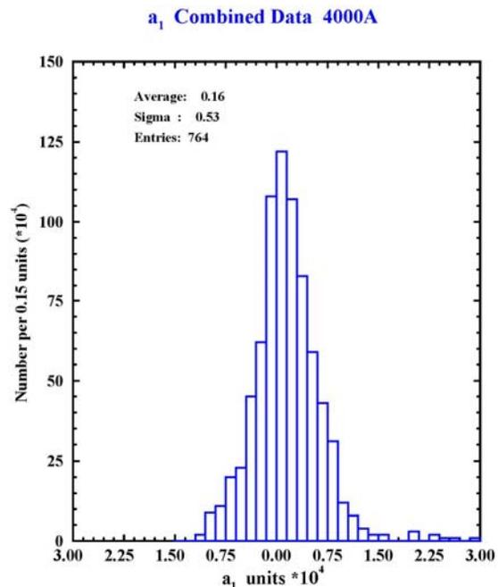
Figure 3 Final distribution of skew quadrupole in Tevatron dipoles after production shimming
