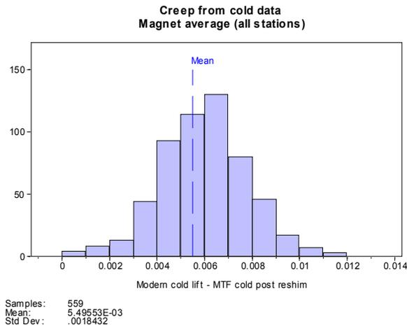
Figure 2 Distribution of lift changes from production to now due to creep. For each magnet the change is averaged over all accessible stations.
