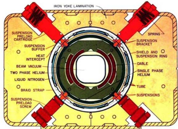
Figure 1 Tevatron dipole cross section
