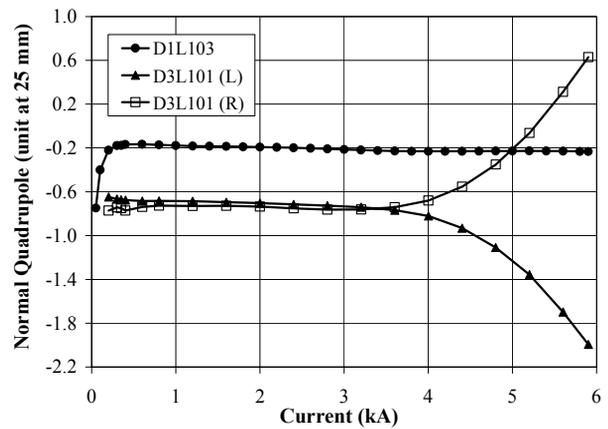
Fig. 3: Variation of the integral normal quadrupole term with excitation in a typical D1 and D3 magnet
