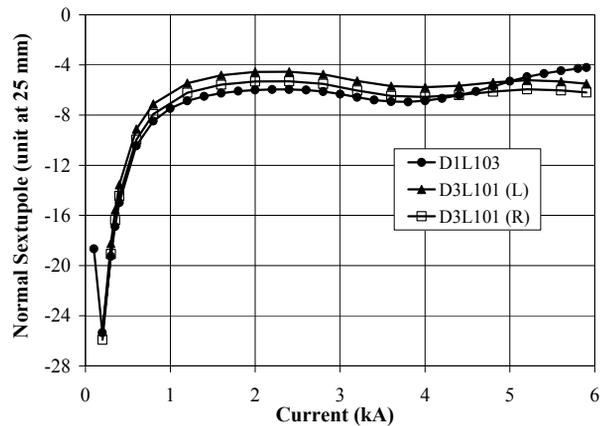
Fig. 4: Variation of the integral normal sextupole term with excitation in a typical D1 and D3 magnet
