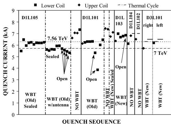
Fig. 1: Quench test results in D1L and D3L dipoles.
