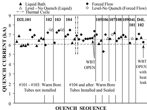
Fig. 2: Quench test results in D2L and D4L dipoles.
