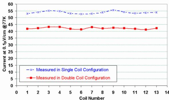
Figure 3: The current at an average voltage gradient of  $0.1 \mu\text{V}/\text{cm}$  ( $10 \mu\text{V}/\text{meter}$ ) over the total length of the coils measured at  $77 \text{ K}$  for the first thirteen pancake coils powered individually and in pairs.
