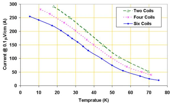
Figure 6: A summary of the temperature dependence of the current in two, four and six coils in the magnetic mirror model. In each case voltage across the coil is closest to the pole tip. Note that the magnetic field is approximately three times as great for six coils as it is for four coils.
