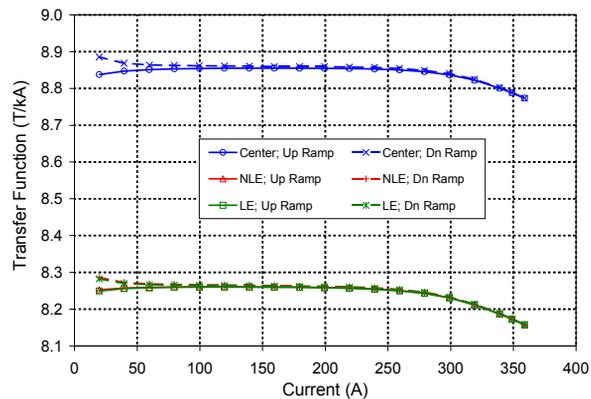
**Figure 6** Excitation curves centered in the different pitch regions, measured with the rotating tangential coil.
