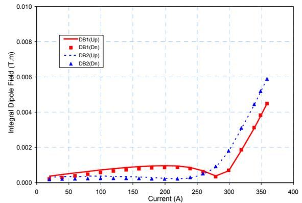
**Figure 7** Integral dipole field measured with two different windings of a full-length rotating coil. The maximum integral value is well below the limit of 0.01 T.m.
