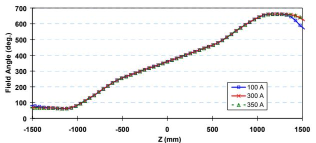
**Figure 4** The angle of the field along the length of the magnet. The center region pitch is  $\sim$ half that in the ends.
