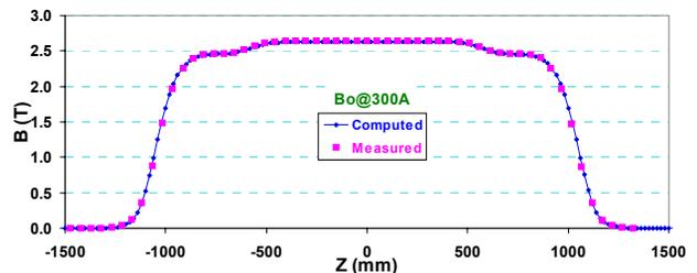
**Figure 3** Field in the magnet along its length. The field is lower in the region of greater pitch.
