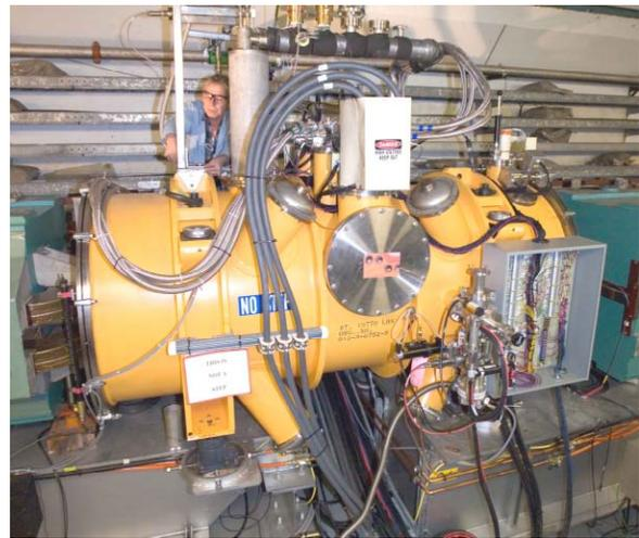
**Figure 8** A photo of the completed snake magnet installed in the AGS ring (Section A20). The cryocooler head connections are behind and to the left of the white box in the top center.
