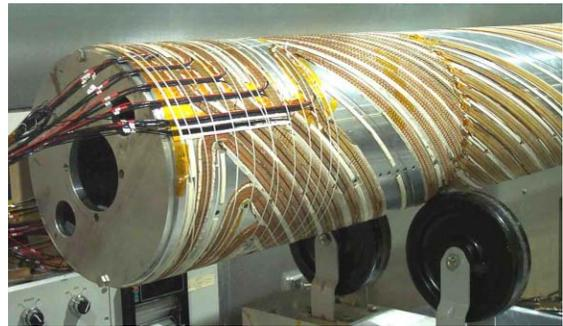
**Figure 1** Photo of the inner coil. The various windings were complete but filler epoxy had not yet been applied.
