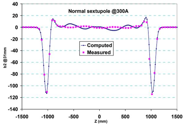
**Figure 5** The sextupole component measured stepwise with a tangential measuring coil 51 mm long,  $r=34$  mm.
