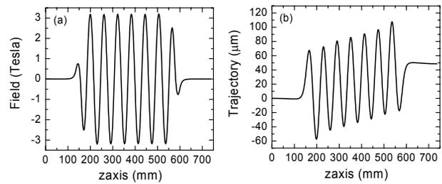
Figure 4: Field measurement in the vertical tests dewar (a) magnetic field distribution and (b) second field integral distribution.
