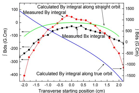
Figure 1: Field integral along the true and straight orbit starting from different transverse positions. Solid and dashed lines are the calculated and measured field integral, respectively.
