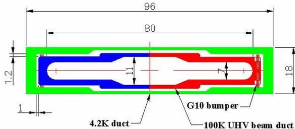
Figure 2: Cross-section of aluminum UHV beam duct and 4.2 K vessel aperture duct (unit: mm).
