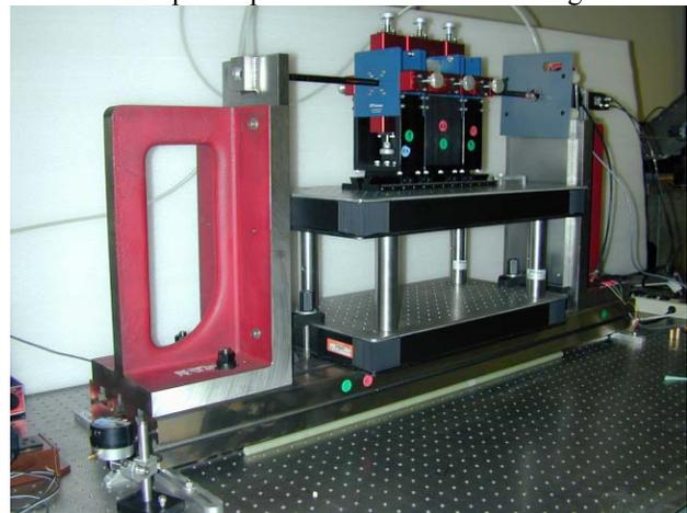
Figure 1: Air Bearing Rotating coil system. A triplet is being measured.
