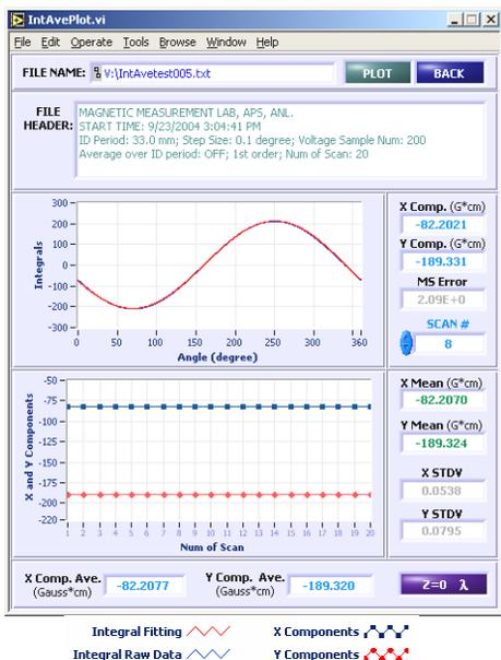
Figure 2: Earth magnetic field integral measurements.
