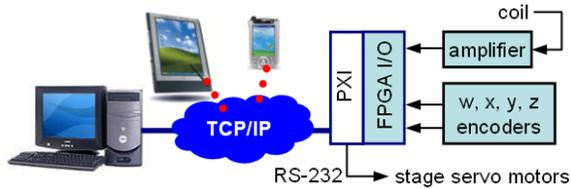
Figure 1: System control and data acquisition architecture schematic layout.
