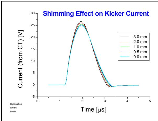
Figure 5: The shimming effect on the change of current waveform.
