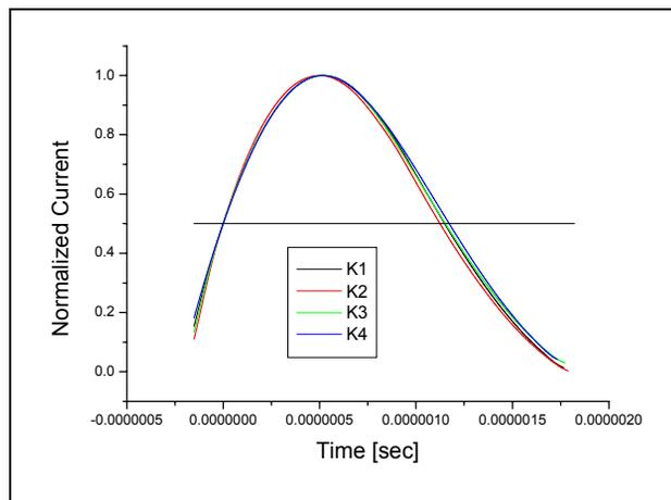
Figure 4: Mismatch of four kicker waveform.
