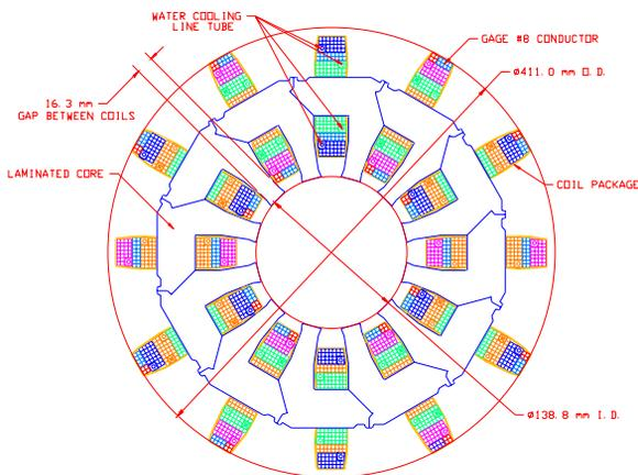
Figure 2: Corrector with indirect water-cooling.
