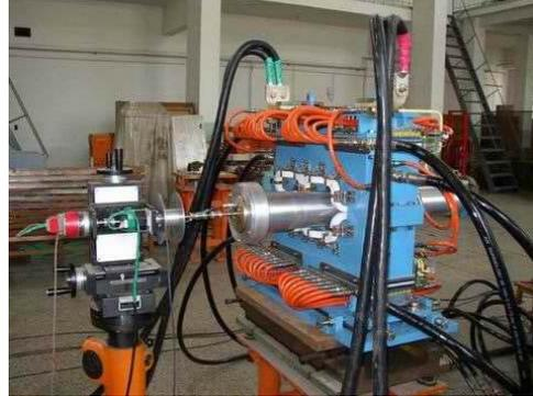
Fig. 5 Harmonic measurement of Q1a
