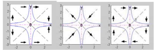
(a) For  $b_{3n}$  shim (b) for  $b_{4s}$  shim (c) for  $b_{6s}$  shim
