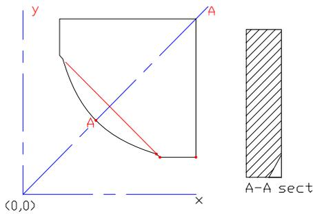
Fig. 8. The optimum shape of Q1a end chamfer
