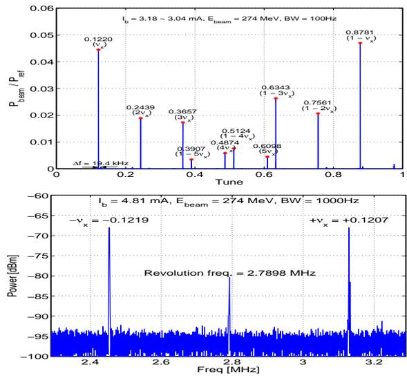
Figure 2: Measured betatron and synchrotron spectra of a hollow beam in a 274 MeV lattice with a horizontal chromaticity  $\xi_x = -0.45$ . Upper plot: measured betatron tune spectra which show the aggregated data from five consecutive measurements. Lower plot: measured synchrotron spectrum.
