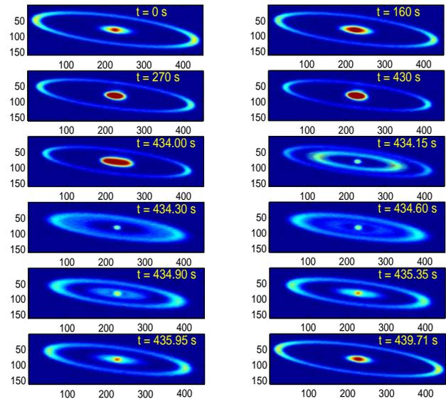
Figure 3: A series of images captured at various of times during a cycle of beam evolution. All images are plotted using the same intensity map. Single bunch current decreases from 0.558 mA at  $t = 0$  s to 0.545 mA at  $t = 440$  s.
