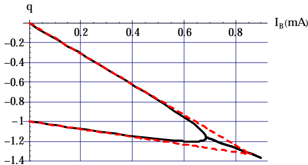
Figure 6: TMCI threshold for a bunch current. Two-mode model.
