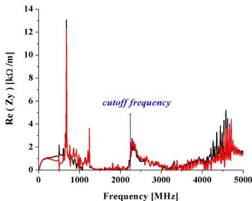
Figure 5: The vertical impedance of SC rf cavity simulated by the rf code GdfidL. The vertical beam offset is 15 mm for the black line and -15 mm for the red line respectively. The cutoff frequency of transverse waveguide mode in the beam pipe is 2.237 GHz.
