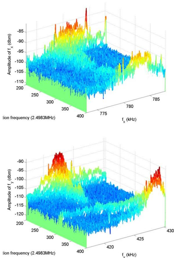
Figure 4: The spectrum of transverse BPM signal measured in user operation. The beam current was 180 mA and the transverse feedback was turned on. The top graph is the spectrum of horizontal BPM and the bottom is the one of vertical BPM.
