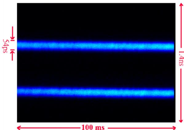
Figure 3: The longitudinal bunch motion measured by a streak camera. The total beam current is 200 mA and the fill pattern is uniform. The measured rms bunch length is 22 ps. The revolution period of TLS storage ring is 400 ns.
