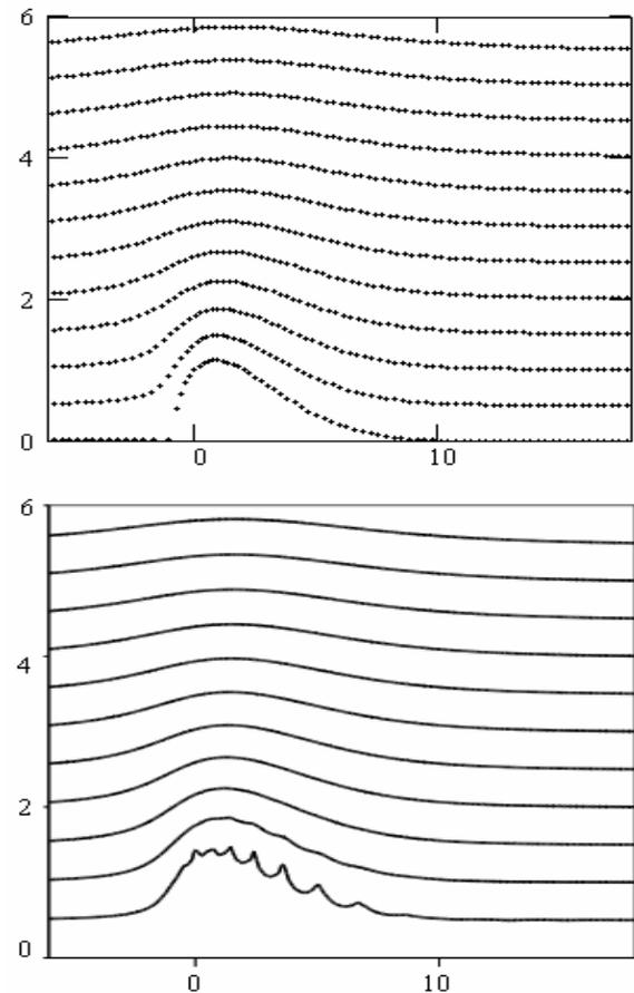
Figure 2: The lines of equal maximal growth rates on the complex plane of the variable  $\lambda = A \sum_m m Z_m (-i\Omega - im\omega_0)$ , obtained with the approach of short bunches (above) and with the method of present paper, for approximation orders  $k_{max} = 40$  (below).
