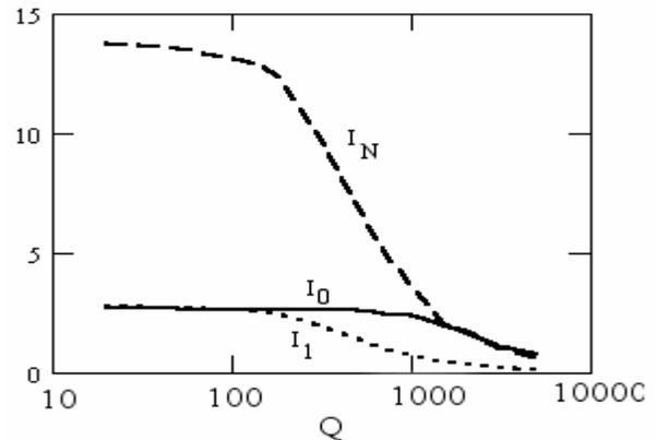
Figure 1: The dependence of the threshold current of the whole multibunch beam  $I_N$ , of its one bunch  $I_1$  and of the singlebunch beam ( $I_0$ ) on the quality factor  $Q$ .
