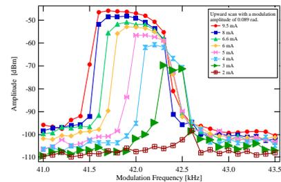
Figure 2: Example of measurement of the synchrotron line amplitude as a function of the stored current in a single-bunch.
