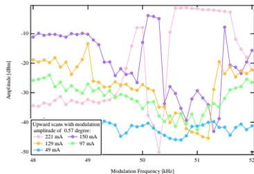
Figure 4: Frequency scans in multibunch mode as a function of stored current.
