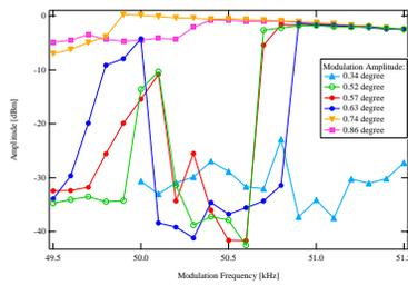
Figure 3: Behavior of the synchrotron line for different modulation amplitude in multibunch mode. Measurement done with 200 mA and gap voltage of 500 kV.
