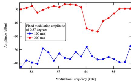
Figure 6: Simulation results of the amplitude of the excited dipolar oscillations in multibunch mode with two different values of stored. The accelerating voltage used was 500 kV.
