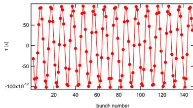
Figure 1: Phase relation between bunches caused by the presence of the longitudinal CBM 133.
