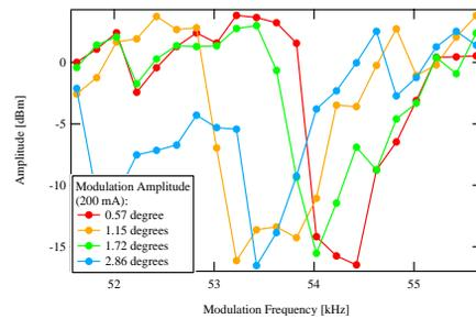
Figure 5: Simulation results of the amplitude of the excited dipolar oscillations in multibunch mode with different modulation amplitudes. The accelerating voltage was 500 kV and the current 200 mA.
