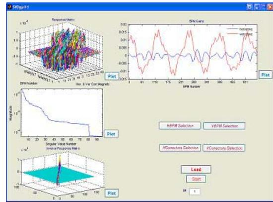
Figure 2: GUI using MATLAB Accelerator Toolbox for global orbit feedback.
