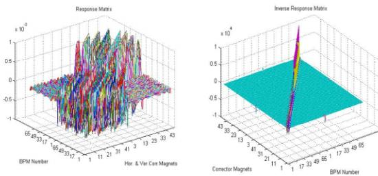
Figure 3: Response (left) and the inverse (right) matrixes of the CANDLE storage ring.
