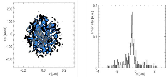
Figure 6: Photon beam phase pattern (left) and intensity profile (right) produced by electron beam after focusing by CRL (10 keV).
