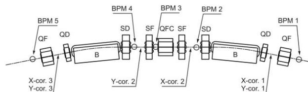
Figure 1: BPMs and correctors distribution per magnetic lattice.
