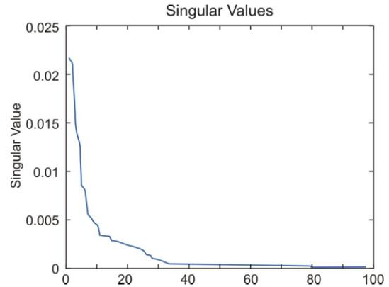
Figure 4: Singular values of the response matrix.
