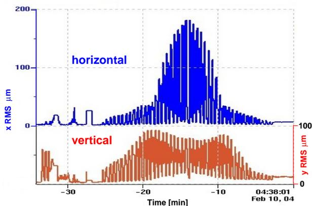
Figure 2: Horizontal and vertical RMS orbit response of all DPMs during IDFF recording for one of two electromagnetic undulator UE212 at the surface/interface spectroscopy (SIS) beamline. Applying the estimated correction after each IDFF step restores the original RMS values within a few  $\mu\text{m}$  (see comb like shape). This IDFF table generation for one ID parameter takes  $\approx 20$  min. The FOFB is switched off during the entire measurement.
