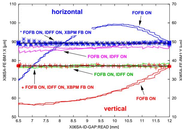
Figure 3: Stabilization of the horizontal and vertical photon beam position at the XBPM of a protein crystallography (PX) beamline  $\approx 8.6$  m away from the source point of the in-vacuum ID **U24** during gap variations at a speed of 0.1 mm/s by means of FOFB, FOFB + IDFF tables and FOFB + IDFF tables + XBPM feedback.
