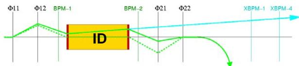
Figure 1: Illustration of the ID feed forward correction scheme (IDFF). The analogue Bergoz BPMs (ABPMs) “BPM-1/2” and the slow correctors at  $\Phi_{12/21}$  are not included in the FOFB loop whereas the fast correctors at  $\Phi_{11/22}$  as well as the XBPMs are integrated in the FOFB.
