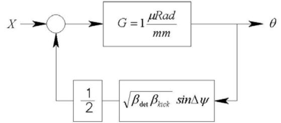
Figure 1: the schematic of the feedback loop.
