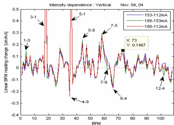
Figure 3: The linear change of vertical position reading of 108 BPMs per 1-mA beam current change. The blue line corresponds to the beam current change between 112 mA and 153 mA, the green line between 153mA and 188mA, the red line between 112 mA and 188mA.
