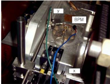
Figure 4: Linear voltage displacement transducers installed on the vacuum chamber near BPM. X denotes the horizontal position sensor and y the vertical direction.
