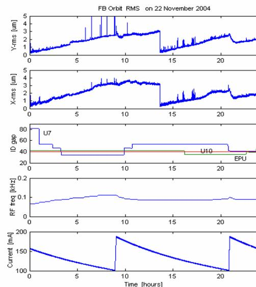
Figure 1: The orbit data for one day under orbit feedback. The first graph: vertical orbit RMS, the second: horizontal orbit RMS, the third: insertion device gap, the fourth: RF frequency, and the last: beam current.
