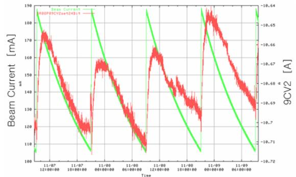
Figure 6: The change of corrector current under the orbit feedback for two days. The red line: corrector (9CV2) current, the green line: beam current.
