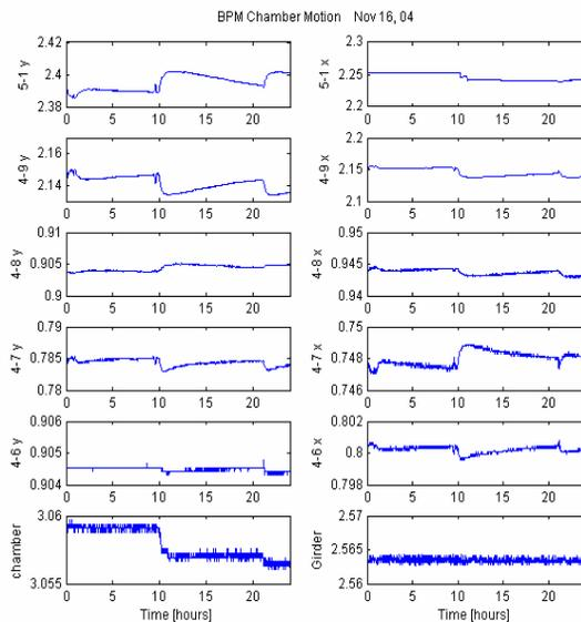
Figure 5: The measured vacuum chamber motion as the stored beam current changes for one day. The vertical scale in each figure is mm. The first number in the name of BPM 5-1y represents the cell number, and the last the BPM number in that cell.
