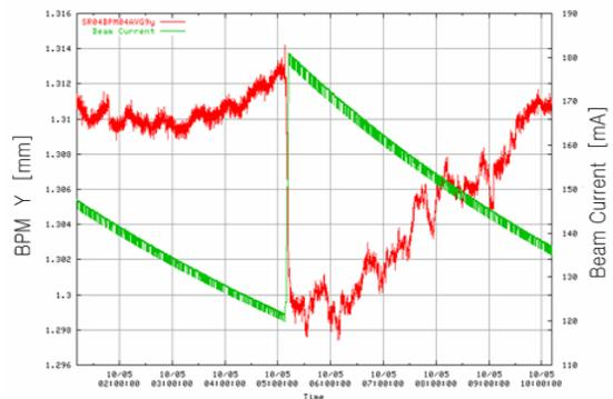
Figure 2: The vertical BPM reading change when the beam is re-filled. The red line: BPM reading, the green line: beam current.
