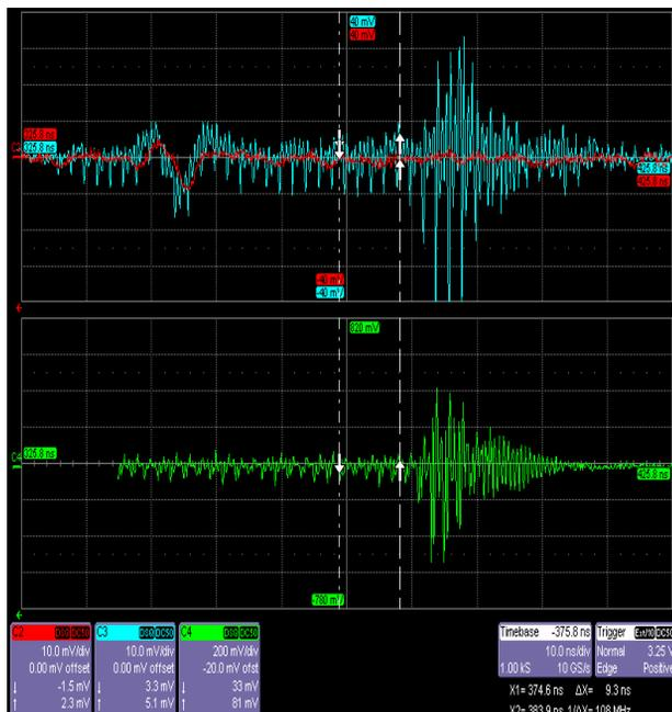
Figure 4: Feedback, kicker (upper part) and filling pattern detected by the ring electrode (lower part) signal as seen on the oscilloscope. For purpose of feedback adjustment the machine was filled with only 3 bunches.
