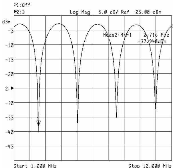
Figure 3: Frequency transfer function of the notch filter. Revolution frequency (2.72 MHz) and three harmonics of the filter are shown.
