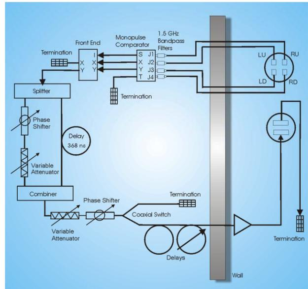
Figure 1: Layout of the analog vertical feedback.
