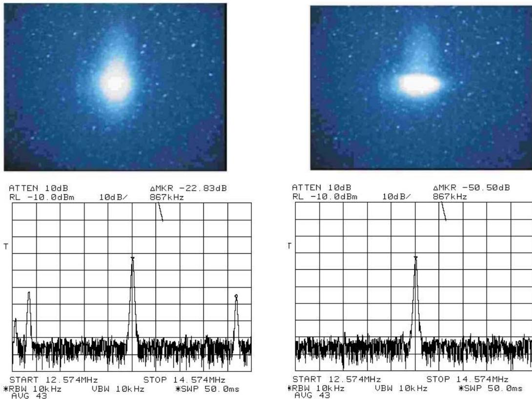
Figure 5: Synchrotron beam profile (upper part images) and frequency spectrum (lower part plots) without (left) and during (right) feedback operation. Note that sidebands vanish completely when TFS is in use.
