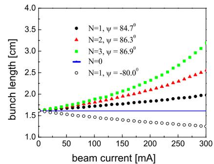
Figure 2: Bunch length versus the beam current for different  $N$ , the number of the harmonic cavities. They are calculated by (16) and are compared with the solid line that is calculated by (17).
