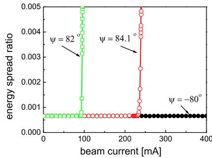
Figure 1: The energy spread ratio at different tuning angle for the currents, which are below and over the threshold of the Robinson instability. The number of the harmonic cavity is one. The bunch number is one.
