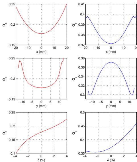
Figure 4: Tune shift versus horizontal amplitude (top), vertical amplitude (middle) and energy (bottom). The chromaticity is corrected to (1,1)
