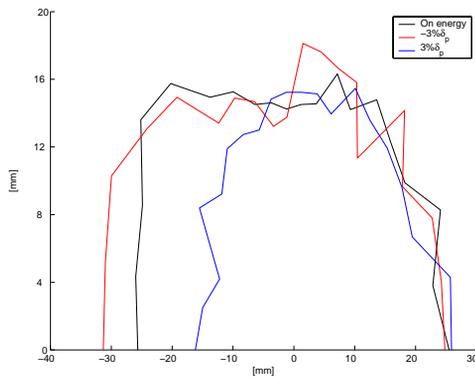
Figure 3: Dynamic Aperture at the center of the long straight section for injection ( $\beta_x = 10.8$  m,  $\beta_y = 5.7$  m), for the on-momentum particle and for particles with  $\pm 3\%$  energy deviation for the ideal machine. The particles are tracked for 400 turns. The effect of the chromatic closed orbit is included.
