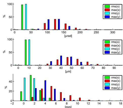
Figure 2: Statistics for 1000 sample machines, applying errors of  $100 \mu\text{m}$  in the girder position and of  $60 \mu\text{m}$  in the element respect the girder position. Bottom graph shows the statistics of uncorrected orbit, middle graph the ones of the corrected orbits, and top graph the ones of the correctors. The correction has been performed using SVD with 90 eigenvalues out of 120.
