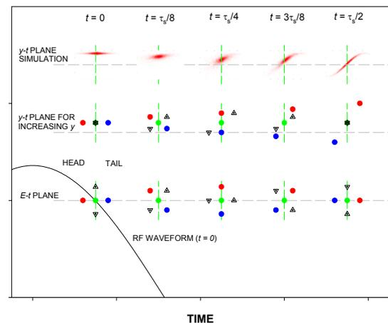
Figure 1: Illustration of an electron beam's synchro-betatron motion in a ring with positive chromaticity: (bottom row) longitudinal phase space motion of four electrons initially at the extreme ends of energy / time scale; (middle) motion of the four particles in  $y$ - $z$  plane; and (top) collection of  $10^4$  electrons in  $y$ - $z$  plane.
