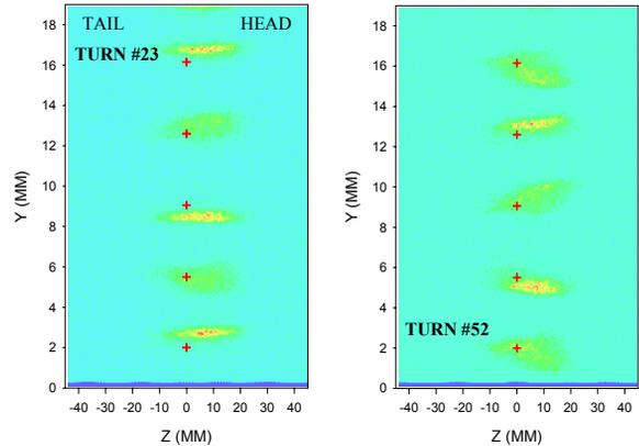
Figure 4: Side-view streak images of with turn indices (left) No. 23 to 27, and (right) No. 47 to 52.
