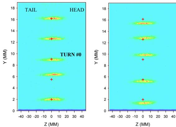
Figure 3: Side-view streak images of the stored beam probed by a vertical kicker. The turn indices are (left) No. -2 (top) to +2, and (right) No. 3 to 7.
