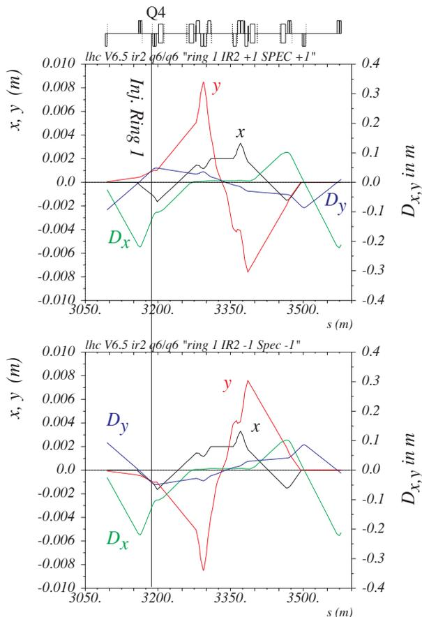
Figure 2: Orbit and dispersion for positive (top) and negative (bottom) vertical crossing angles at IR2.
