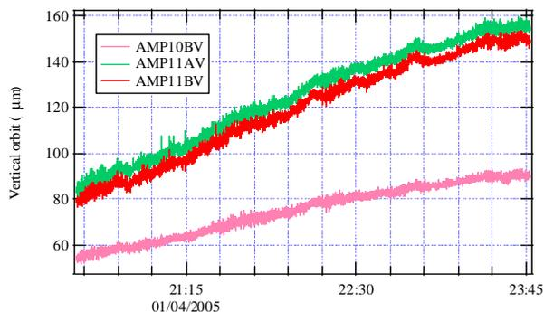
Figure 4: Example of matched readings for a pair of BPMs in the same shielding box (AMP11A and AMP11B).
