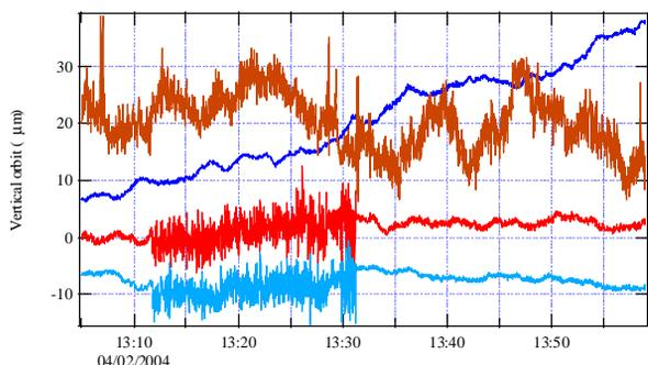
Figure 2: Examples of altered noise level affecting individual and group of monitors. Beam with no orbit correction.
