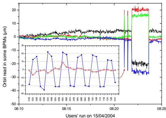
Figure 1: 6-fold symmetric horizontal orbit variation due to interaction with a HOM in the RF cavity.
