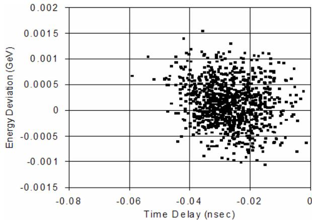
Figure 11: Phase Space distribution after the debuncher cavity given the linac output energy error in Figure 5.
