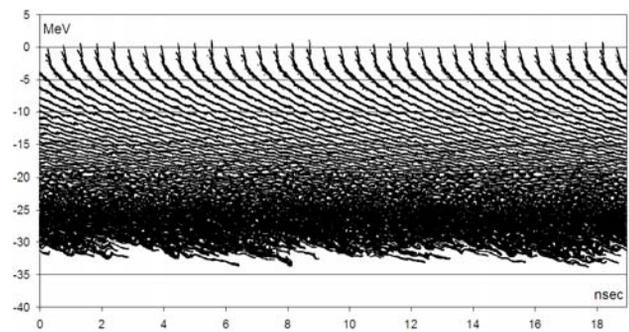
Figure 13: Preliminary calculation of energy spread growth in the Main Injector over the 270 turns of injection.
