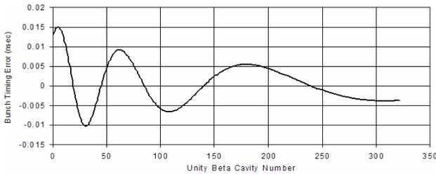
Figure 4: Propagation of SNS level phase and energy jitter from 1.2 to 8 GeV leading to maximal output phase error.
