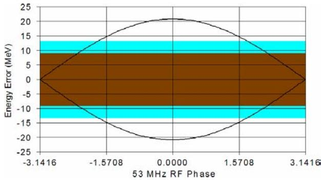
Figure 9: The dark (brown) shaded area is the output 95% energy spread of the Proton Driver when jitter is fully compensated. Note the no other correction is necessary.
