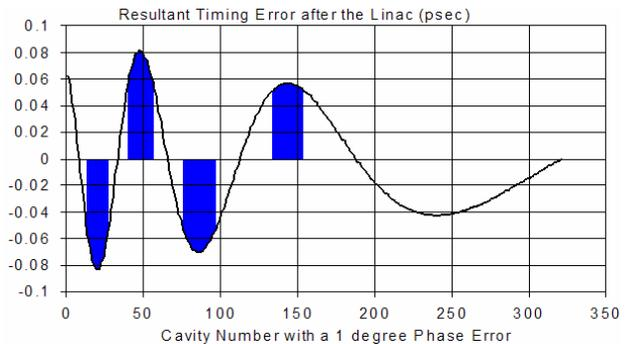
Figure 7: Timing (phase) correction per cavity upon a one degree change in the phase of that cavity.
