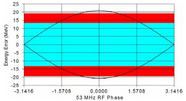
Figure 6: Beam energy width (total shaded area) out of the proton driver assuming SNS emittances and jitter levels.
