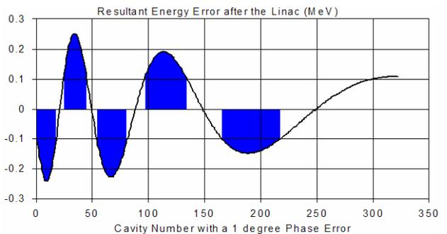
Figure 8: Energy correction per cavity upon a one degree change in the phase of that cavity.
