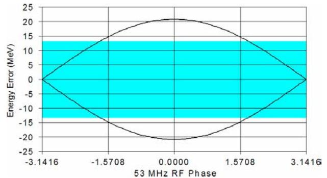
Figure 1: Phase space area of a 0.5 eV-sec RF bucket at injection in the Main Injector, along with the same area for a fully debunched beam (shaded area).
