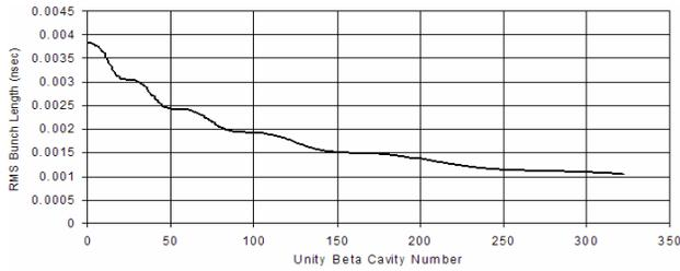
Figure 2: Calculated reduction in bunch length during acceleration from 1.2 to 8 GeV assuming SNS longitudinal emittance and no jitter errors.
